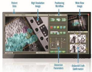
Following the vision system's identification of the optimal hair follicles for transplant, the ARTAS® System dissects these follicles using a sharp needle to score the epidermis and a punch, coaxial with the needle, to separate the graft from the surrounding tissue. In the final step of the harvesting phase, the grafts are removed manually with forceps by the physician or the technician. The grafts are then cleaned, inspected and prepared for implantation.
